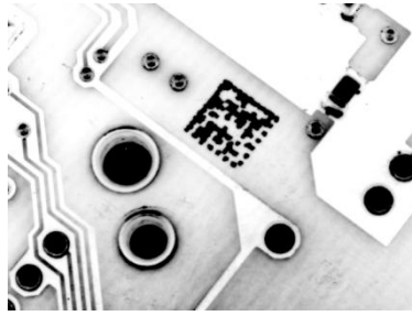
Figure 22 - Data Matrix Code Directly Marked on PCB Surface by Using Laser Etching Technology
