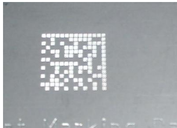
Figure 19 - Dot Peening Marking on Metal Surface with Multi-dot per Code Element
